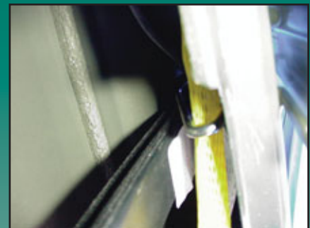
3. The TT-1001 tool hooked around the inside lock control linkage.
